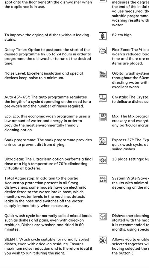
The Aquatest sensor is an electronic sensor that measures the degree of water transparency at the end of the initial soaking phase. ased on the values measured, the sensor sets the most suitable programme, thus obtaining the best washing results with the minimum amount of water.
